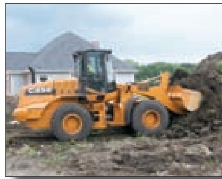
use the wheel loaders to scrape away the material and load it onto a truck. They also use the wheel loaders for hauling away asphalt from road projects for recycling.
