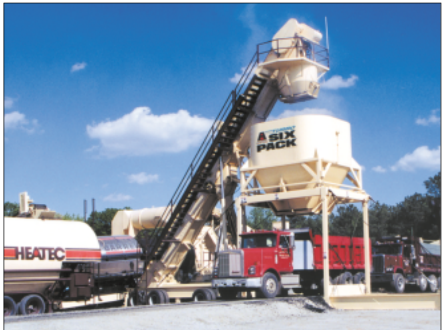
An Astec Six Pack asphalt plant is completely portable, with built-in running gear, and is fully self-erecting. It can be taken down, moved and set up again in 36 hours. Pictured is a truck waiting to receive HMA from the hopper and a silver Double Barrel drum mixer.
