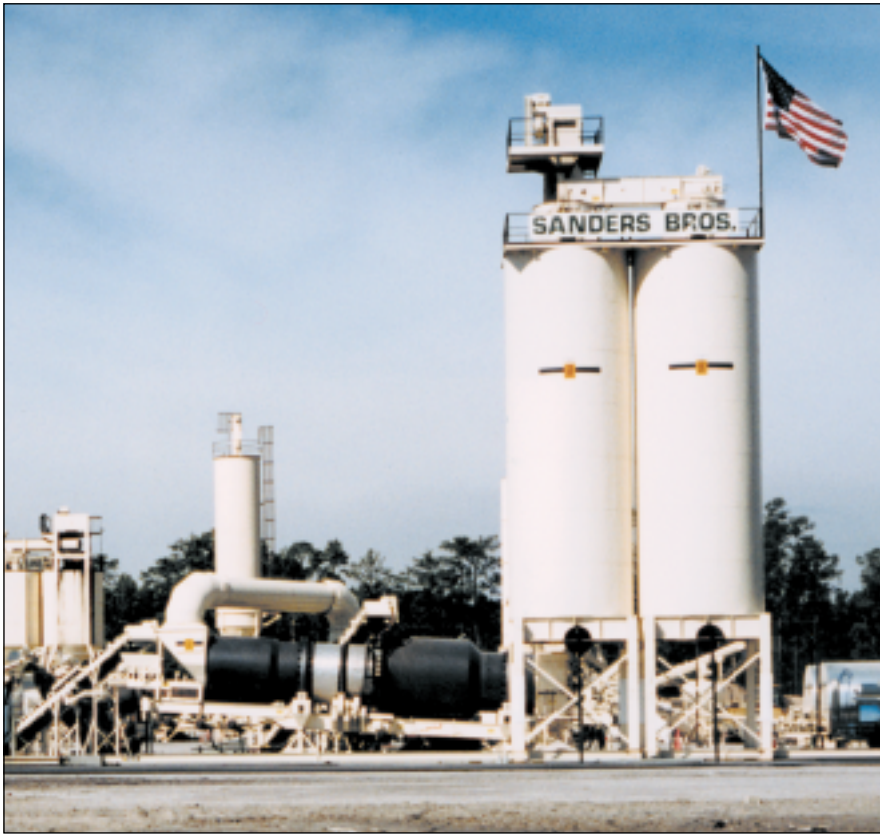
CMI's Triple-Drum combines three distinct drying and heating zones in a single drum.
