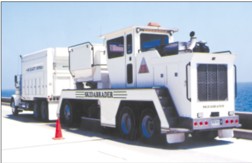
The Skidabrader handles the job of texturing the surface of concrete.
