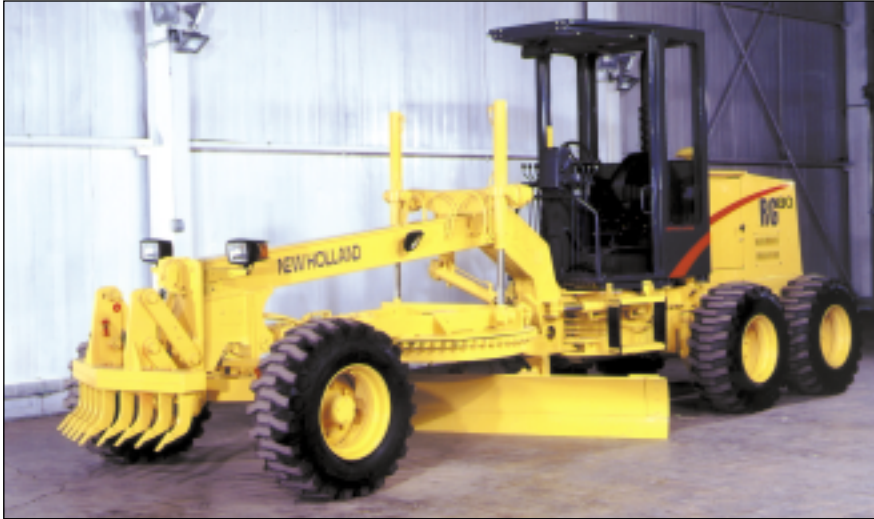
New Holland's two brand new motor graders—the RG80 and RG100—feature a long wheel base for increased stability and articulation for maneuverability.
