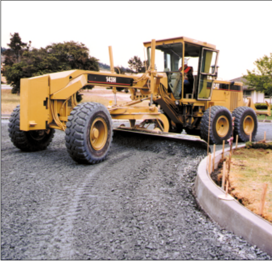
Caterpillar's 143H comes with a turbocharged diesel engine that produces 185 hp.
