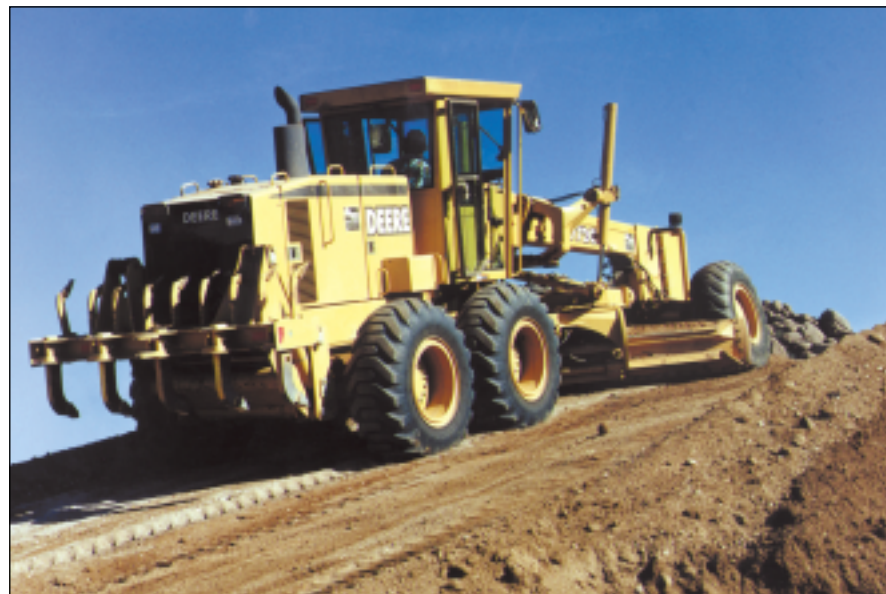
Deere's C Series motor graders feature the PowerShift Plus direct-drive countershaft transmission, which was built especially for the C Series.
