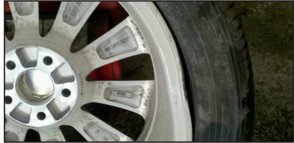
An example of rim and tire damage caused by a raised manhole.
