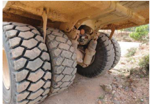
Don't Do This: 4 different tires are mounted on the rear axle of this haul truck; some are new, some are worn and tread patterns and brands are mismatched.
