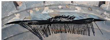
Zipper-like injury resulting from running tire under-inflated.
