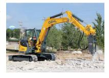
and flow. Edge breaker models also are available for use on mini excavators. The skid-steer-loader models come standard with hoses, a hose saver kit and flat-faced couplers. The model's nitrogen-charged back head increases impact energy, and the absence of through-bolts decrease maintenance times. The breakers' advanced hydraulic circuit provides increased flow to the valve and piston, resulting in faster cycle times and increased tool penetration.
