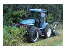
with a cutting width of 80 in. It can be attached to tractors with up to 260 PTO horsepower and a Category II or III three-point hitch. Depending on the type of operation, the unit can be pushed or pulled behind the tractor to cut, mow or mulch material. The 21-in. rotor is mounted on 3-in. piloted bearings with antiwrap protection, and is available with either fixed teeth or individually mounted hammers, which swing 360° on double-tapered rolling bearings.
