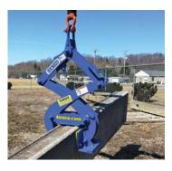
grip range handles a wide assortment of curbing sizes. Rotating pad angles conform to match the wall slope. The elastomer pads provide unmatched gripping performance. The KL1500 weighs 115 lb and boasts a lifting capacity of 1,500 lb. Larger models are available up to 40,000-lb capacities. **Write in 903**
