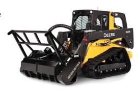
bar helps to topple trees and brush while protecting the carrier from debris. Featuring a two-speed hydraulic system, the MH60C is able to efficiently utilize available horsepower. Preset pressure levels allow the motor to automatically shift to high displacement, increasing torque by 3% to reduce stalling and increase rotor speed recovery. **Write in 904**
