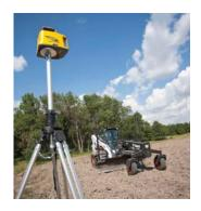
alternative method of automatic grade control on jobsites not suited to lasers. Where usage of a laser requires a flat plane on the jobsite, using a sonic/slope setup allows for going up and down hills while still achieving the correct slope. Bobcat's sensor-kit controls are built directly into the deluxe instrumentation panel on M-Series loaders. **Write in 907**
