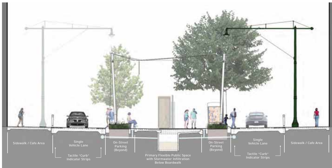
Inverted crown and curbless design were nonstandard elements for this FHWA-funded project. Image courtesy of RATIO Architects Inc.
