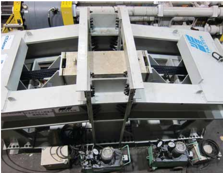
CTLGroup's work in the specialized field of full-scale stay-cable acceptance testing has contributed to the evaluation of better cable design and fabrication practices.
