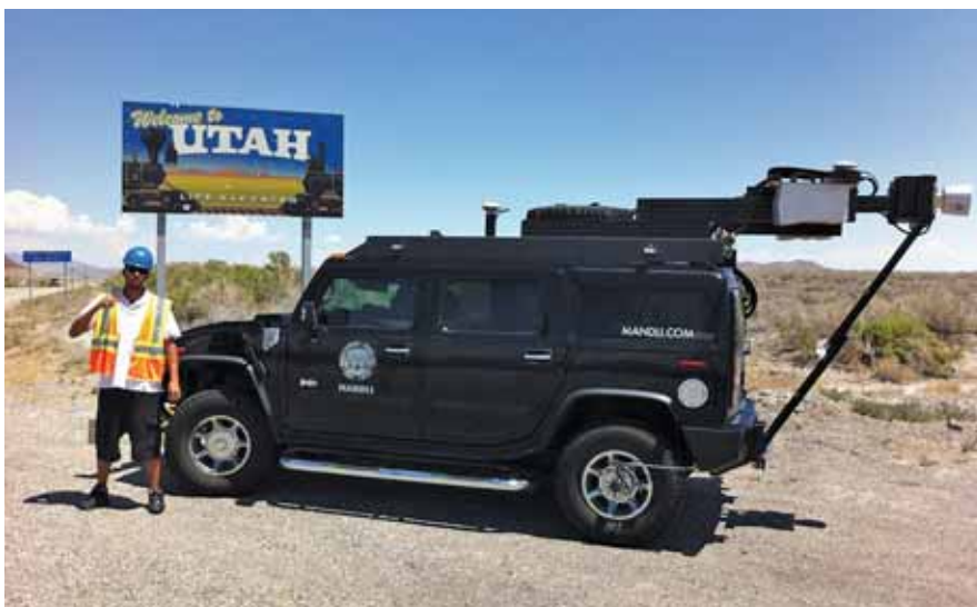
The winning contractor, Mandli Communications, used a mobile platform outfitted with GPS, photolog cameras, a surface profiler, a laser crack measurement system, lidar sensors and a beta version of a sign-retroreflectivity system. Assets were geolocated, categorized and inventoried. UDOT had a rigorous prequalification process for applicants.
