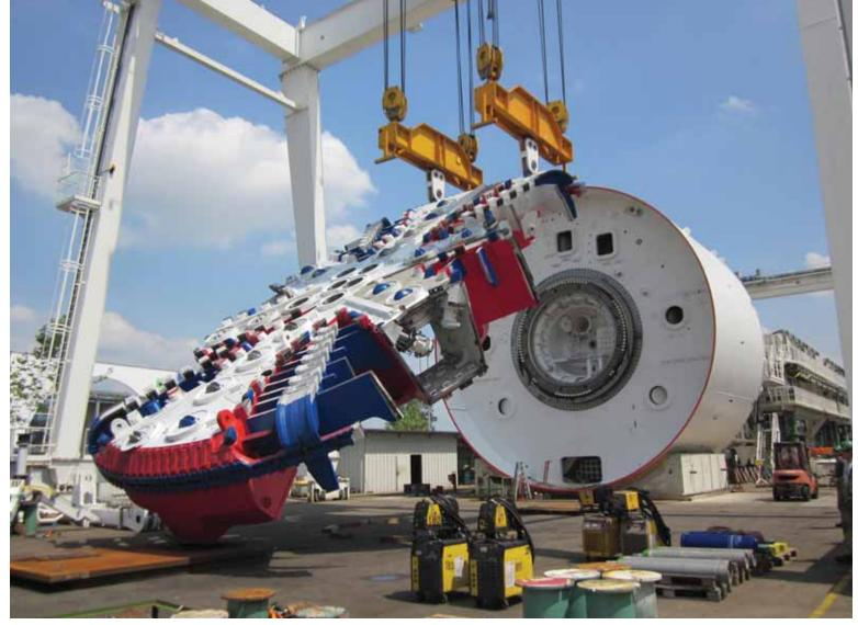
To address this challenge, a slurry-type TBM will be used for excavation. It is critical to the success of the tunnel project that the excavation's face and its full perimeter be controlled at all times to minimize losses of ground and movements of the overlying ground. The mixed-shield slurry TBM will operate in closed-face mode to minimize the possibility of large, uncontrolled ground losses and resulting subsidence.
