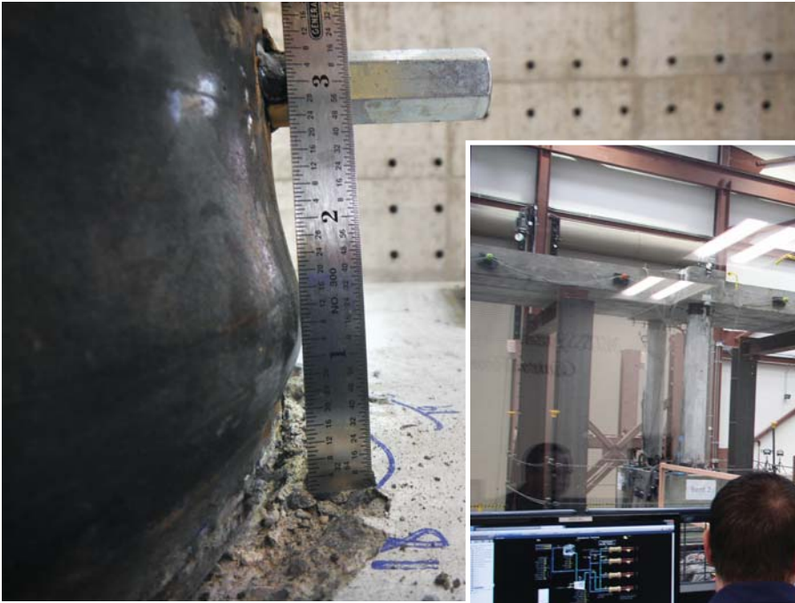
The rocking, pre-tensioned concrete bridge support system is a new bridge engineering design the team has developed with the aim of saving lives, reducing on-site construction time and minimizing earthquake damage.
