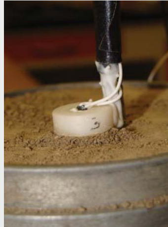
Figure 2. How the Button Heat Pulse Sensor works.
