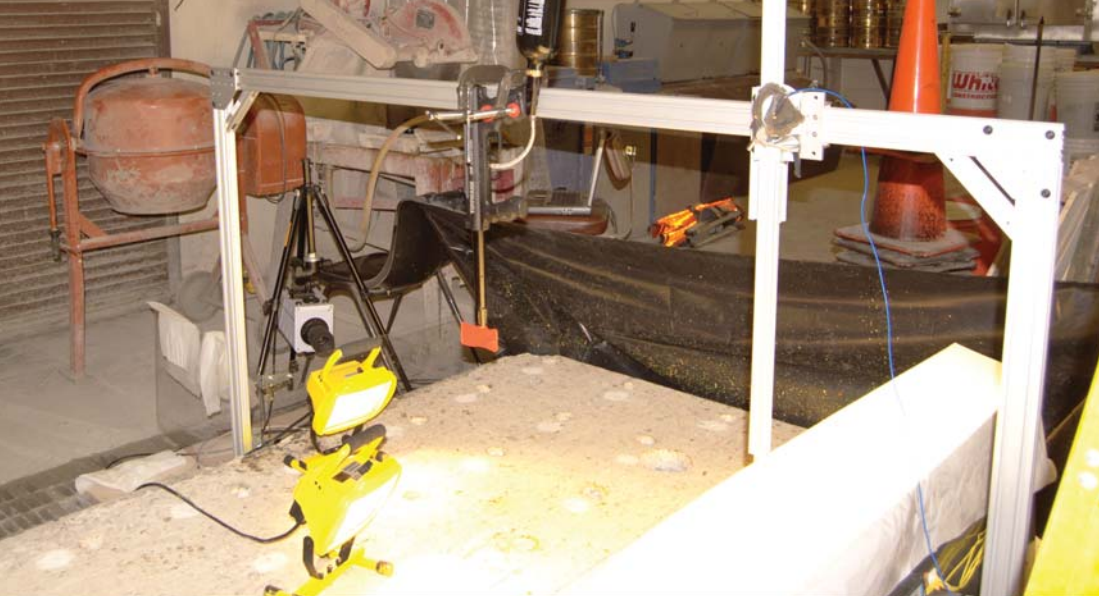
Above left: Brigham Young University laboratory set-up for paintball experiment. The pellets were fired from the suspended gun and their impacts were picked up by ultrasonic microphone (right of picture, taped to the crossbeams).
