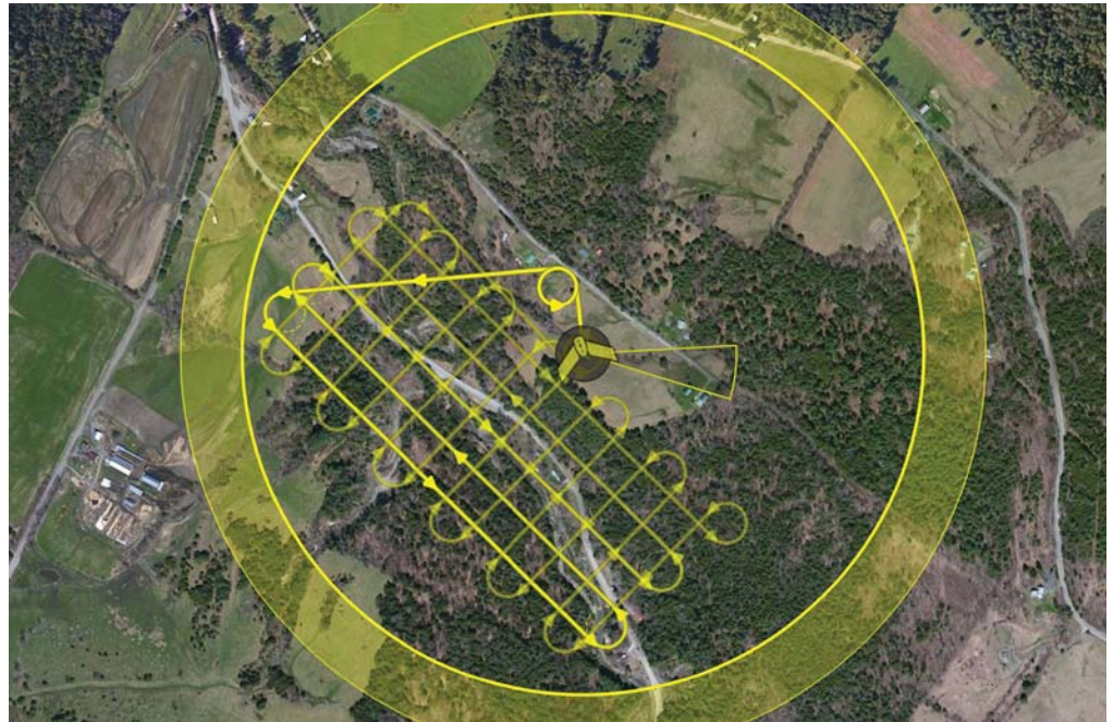
Figure 1. An example flight plan generated for the senseFly eBee UAV via eMotion software.
