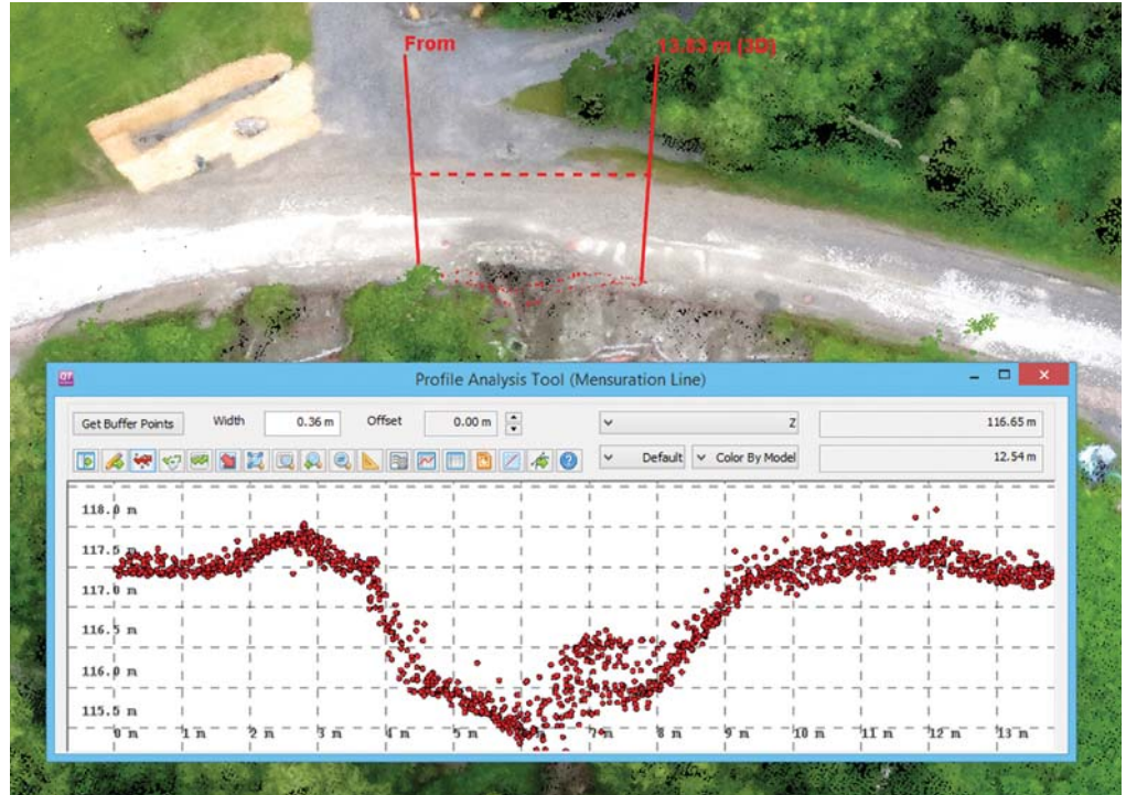
Figure 3. Data generated by UAS imagery of Figure 3's damage site.
