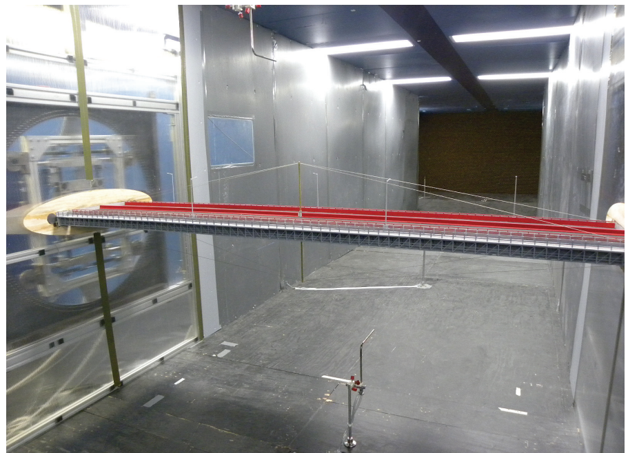
A sectional model of the deck system was tested. The sectional model test procedure focused on the identification of aerodynamic instabilities of the deck involving vertical and rotational motions. To be representative of the full-scale structure, two different modes of vibration with dominant vertical and rotational motions were selected and modeled.
