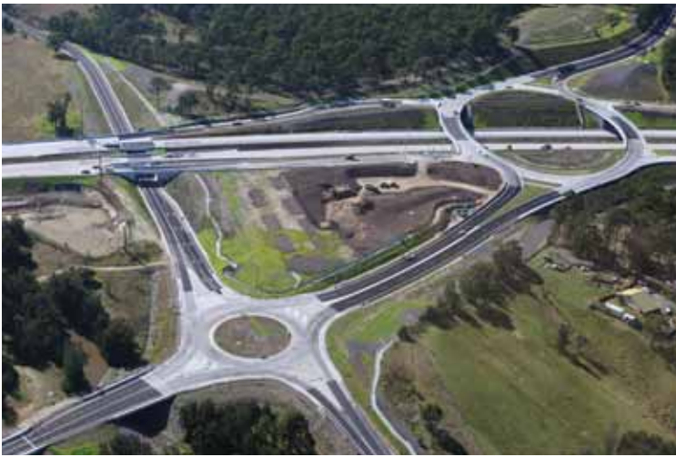
The alignment was shifted through the Sugarloaf Range and the highway elevated over deep gullies to tread more lightly on the landscape and enable wildlife to cross beneath.
