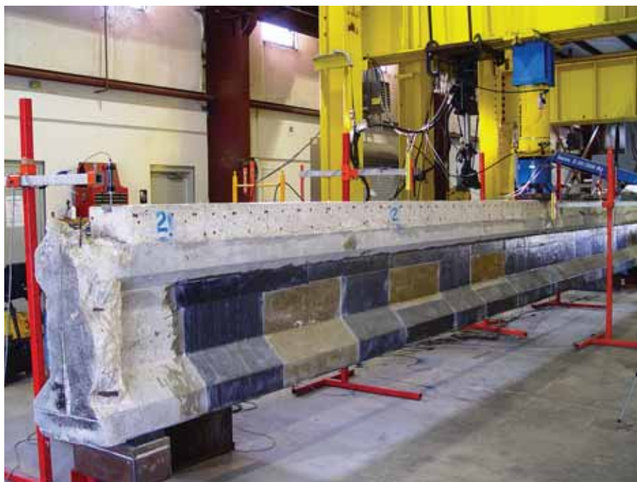
The girders were tested using the hydraulic actuator mounted to a steel frame at mid-span. The fatigue testing of AASHTO II girders was performed using the 110-kip MTS hydraulic actuator selected based on its large-capacity servo valve.
