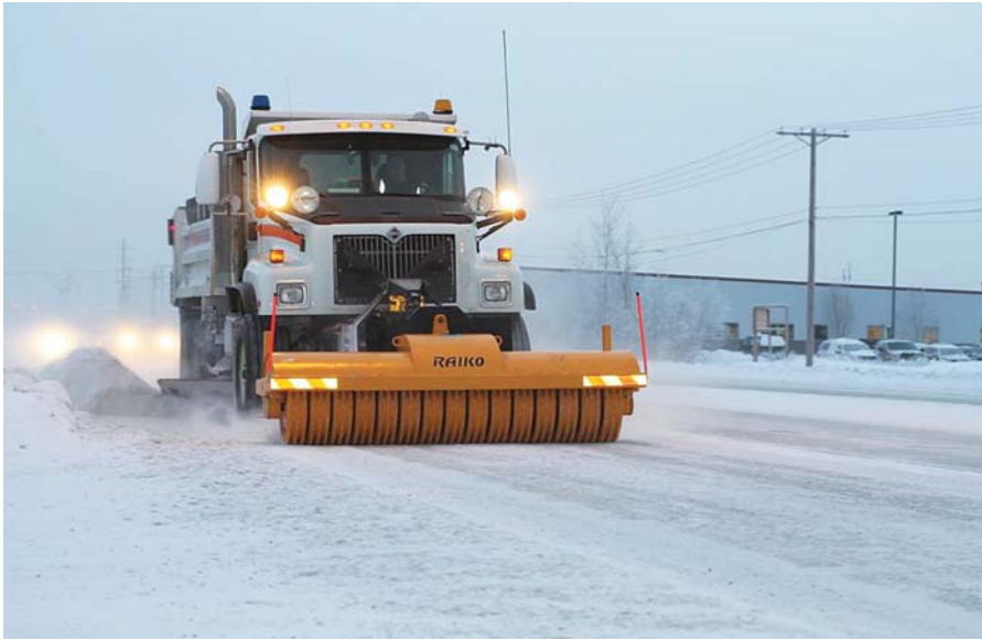
An ice breaker provides a path for chemical deicers to penetrate beneath the ice layer and sever the bond between ice and pavement.
