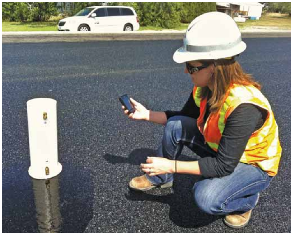
Researchers developed these fine-graded mixes using polymer-modified binders and high-quality aggregates. The mixes themselves must pass both rutting and reflection cracking tests at the design phase. Using good-quality polish-resistant aggregates was key.
