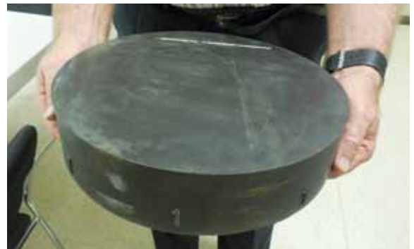
Some 56,000 vibration isolation pucks were installed in the Toronto-York Spadina Subway extension.
